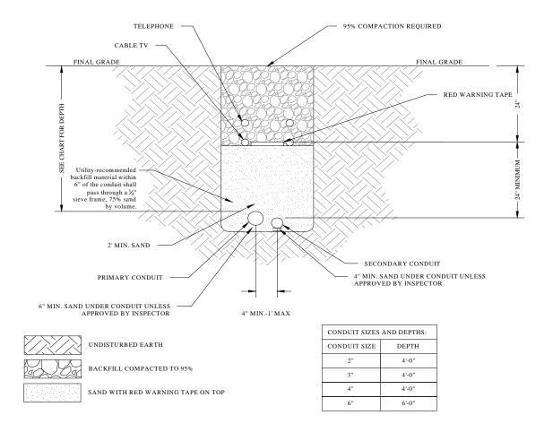
Figure 1 – Trench Cross Section
