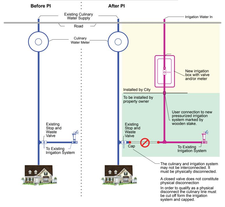
Cross connection of the culinary water system to the pressurized irrigation system is prohibited as it may result in the contmination of the culinary water service and possible fines.
